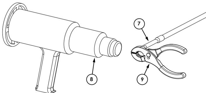
E. Heat the tube "7" by using a heater for heat shrink tubes "8" till the complete shrinkage is achieved and then press the final end of the tube with pincers "9" in order to seal the connection.
