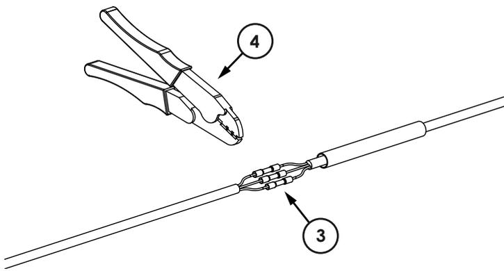
D. Make the connection by using the butt connectors “3”, pressing them with tool “4”
