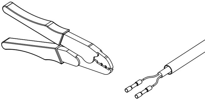
D. Insulate all wires by pressing the butt connectors by a proper tool.
