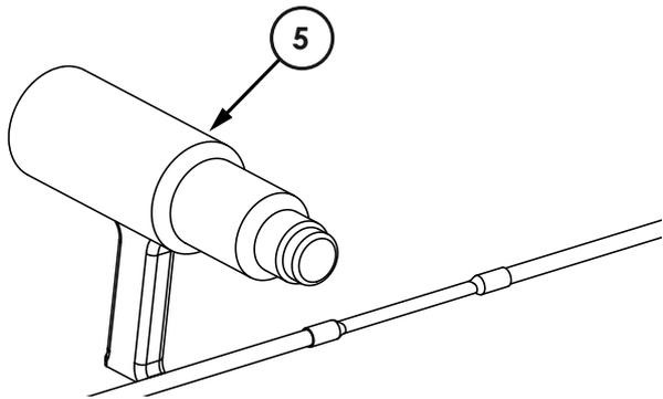
E. Warm up the heat shrink tube by using a heater for heat shrink tubes “5” till the complete shrinkage is achieved. The resulting connection features an IP67 protection rating.
