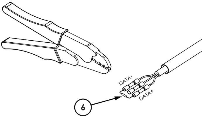
D. Connect the 120  $\Omega$  resistor “6” between DATA- and DATA+ and press the butt connectors by a proper tool.
