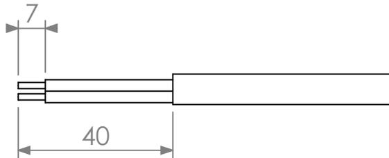
A. Prepare the wires to be connected by cutting and stripping them as shown in the figure.
