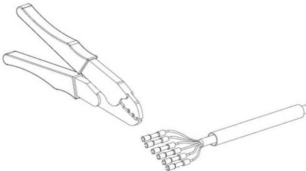
D. Insulate all wires by pressing the butt connectors by a proper tool.
