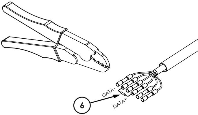
**D.** Connect the 120  $\Omega$  resistor “6” between DATA- and DATA+ and press the butt connectors by a proper tool. Insulate all other wires with the butt connectors.
